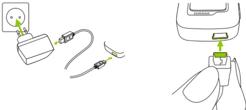
The indicator light is red during charging and will turn green when charging is complete.
